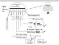
In the drawing, JMP-120R is selection of control signal and ise restrain of RS-485, when there is long distance transmission or noise-control it can short jumper
